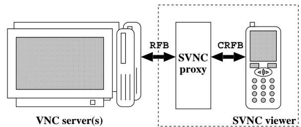
Figure 3. VNC-based architecture
