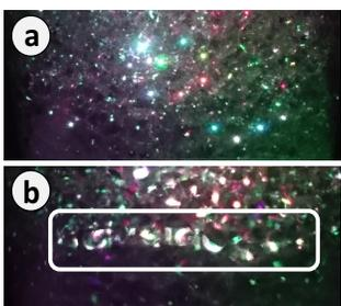
**Figure 5:** Floating-Bubble cloud using an ultrasonic-phased array: (a) non-vibrating bubbles with projection, and (b) vibrating bubbles with projection.
