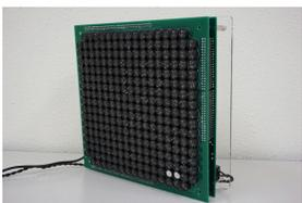
**Figure 4:** Ultrasonic-phased array.
