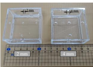
**Figure 6:** Acrylic cases with five holes (scale is  $54 \times 54 \times 24$  cm). Left: hole diameter of 2 mm. Right: hole diameter of 4 mm.
