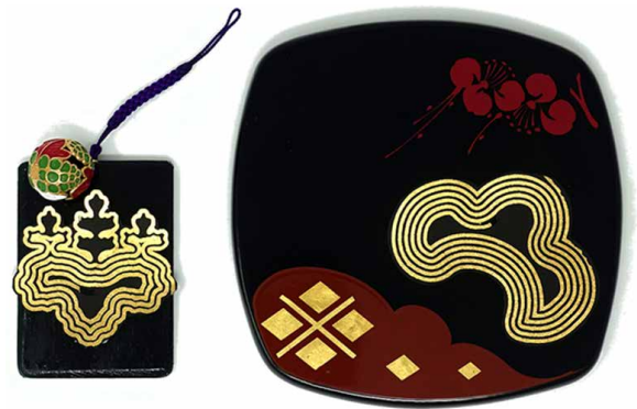
Figure 1: Urushi-ware prototypes with NFC tags whose antennas form Japanese patterns: left) a key chain and right) an ornament. Our method enables designers to embed an NFC tag into an urushi-ware and even decorate it with the tag's antenna in a visually harmonized way with urushi.
