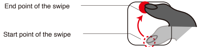
Figure 1: Bounded swipe. In this gesture, the start point and end point of the swipe are inside the target.
