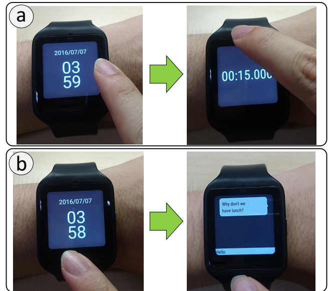
Figure 1. Watch Commander. Users can invoke a function by using B2B-Swipe. (a) Invoking a starting command that starts a timer application. (b) Invoking a starting command that starts a messenger application.
