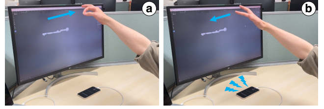
Figure 3: Types of hand gestures: (a) the pinch gesture with the tip of the index finger and the tip of the thumb to draw a line and (b) the gesture other than the pinch gesture to delete a part of an object.
