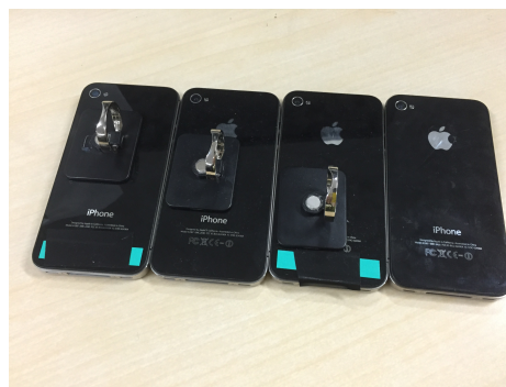
Fig. 2. Ring conditions (from left to right): Top, Middle, Bottom, and NoRing.
