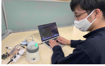
Fig. 1. Actual system setup. Users exchange gaze through the proposed system. When a mutual gaze is established, a voice call starts.
