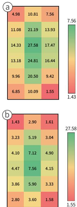
Figure 7: Force-sensitivity characteristic at each touch position: a) non-tape condition. b) with-tape condition.
