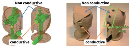
Figure 11: An example of a 3D printed object.
