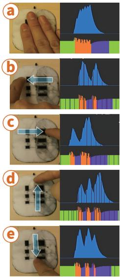
**Figure 6:** Response wave forms (a: tap, b: left swipe, c: right swipe, d: up swipe, e: down swipe). For the purpose of illustration, we only show interactions with the upper row and right column. In fact, all the conductive parts can be used to differentiate gestures.
