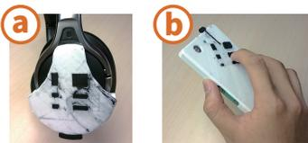
Figure 10: MonoTouch applications (a: headphone cover, b: smartphone case).
