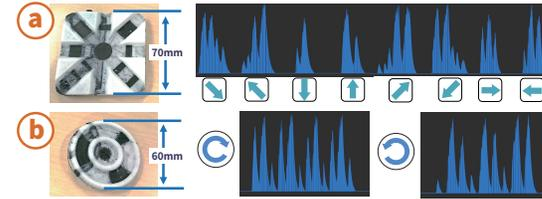
Figure 12: Other examples of electrode layout.
