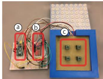
**Figure 5:** Appearance of the structure recognition hardware: (a) arduino Nano, (b) multiplexer, (c) four three-axis Hall sensors.
