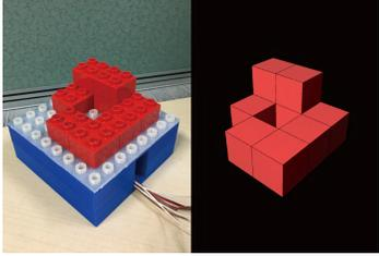
**Figure 6:** Screenshot of our 3D model viewer: (left) structure assembled by the user, (right) the 3D model drawn by the 3D Model Viewer.
