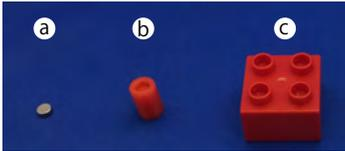
**Figure 3:** Components of the magnetic block: (a) permanent magnet, (b) spacer, (c)  $2 \times 2$  LEGO duplo.
