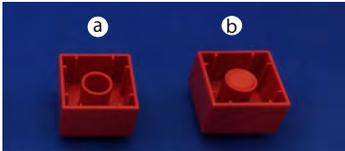
**Figure 4:** The cylindrical cavity inside the  $2 \times 2$  LEGO duplo: (a) cavity, (b) cavity with a spacer inserted.
