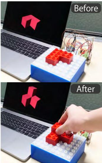
**Figure 2:** Operation example of Tesla Blocks: (upper) before adding a block, (lower) after adding a block.
