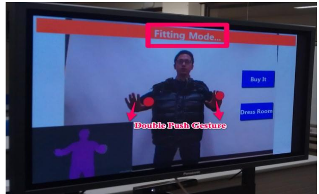
Figure6. Fitting Mode: User uses Double Push Gesture to fit the virtual object with the body.
