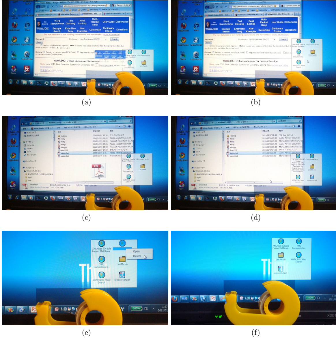
Figure 3.1: Binding and unbinding information: (a) the URL from an Internet browser tab is being dragged and (b) shows the resulting reference list after binding, (c) a pdf file from file explorer is being dragged and (d) shows the resulting reference list after binding, (e) a reference is being deleted and (f) shows the resulting reference list afterward.
