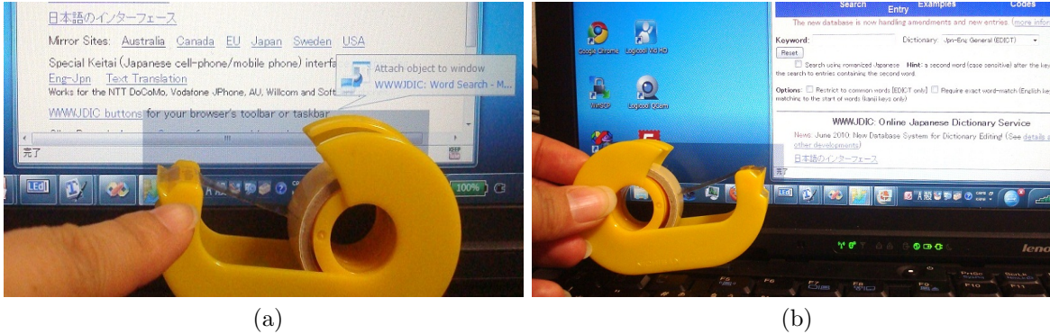
Figure 3.4: Control mode and tracking: (a) switch operation, (b) user is dragging an object in the sensing area.
