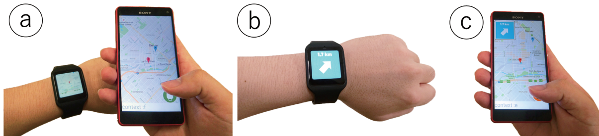
Fig. 1. Map application that demonstrates SynCro's usability. (a) User can use the wide screen of the smartphone to browse the map and select a destination using his or her thumb. (b) After the destination is selected, the smartwatch displays the distance and an arrow to indicate the direction to the destination, which allows for easy viewing while walking. (c) The smartwatch screen is mirrored on the smartphone when the user lowers his or her left arm. The user can then zoom in and out by using a wrist-tilt gesture. The user can use his or her right hand to browse the map again easily and confirm that he or she is walking the proper route.
