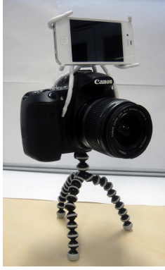
Fig. 1 Prototype of our self-portrait system. A Canon 60D camera is used to take pictures and an iPhone is used as a viewfinder.
