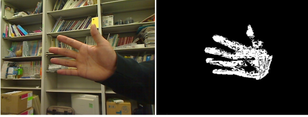
Figure 4. Source (left) and the result (right) after background subtraction and color filtering
