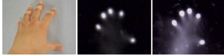
Figure 4. Blobs caused by fingers on the panels. Left: the fingers' posture in this experiment. Center: blobs by the fingers on Silicone Touch. Right: blobs by the fingers on the acrylic panel.
