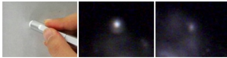
Figure 5. Stylus and blobs by the stylus touched on the panels. Left: stylus of a graphics tablet. Center: blob by the stylus on Silicone Touch. Right: blob by the stylus on the acrylic panel.
