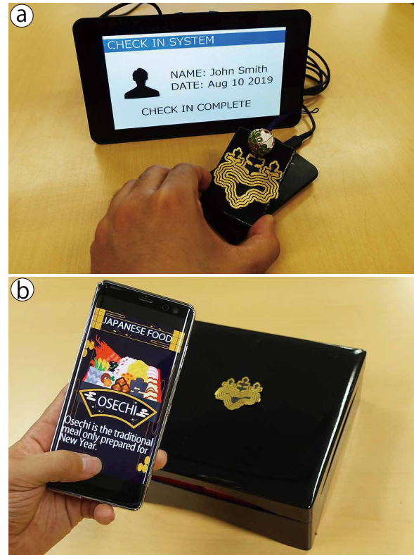
Figure 13: Example applications: a) an IC key tag and check-in application and b) an interactive lunch box that has the information about the meals inside it.
