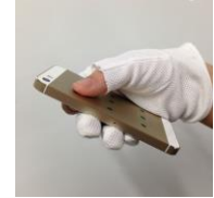
Figure 7: Back condition: The user touches protrusions with his/her thumb, and the touchscreen with his/her index finger.
