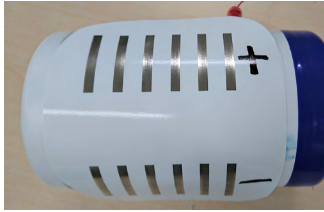
Fig. 10. Personalized controller made from SilverCodes. The user can control the volume by swiping a finger over the identifiers.
