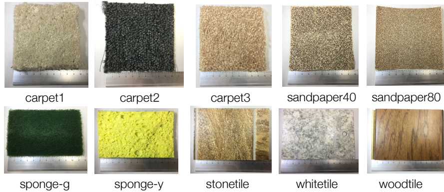
Fig. 4: Textures. These are plate-like object with length 70–100 mm and width 100–130 mm.
