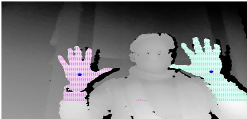
Figure 3. Hand tracking with k-means clustering
