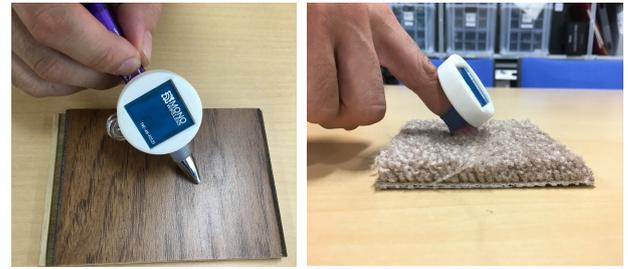
Fig. 4: Collection of tactile data. Put the microcomputer in the 3D printed case, attach it to experimenter's finger or pen and operate it to collect the data.
