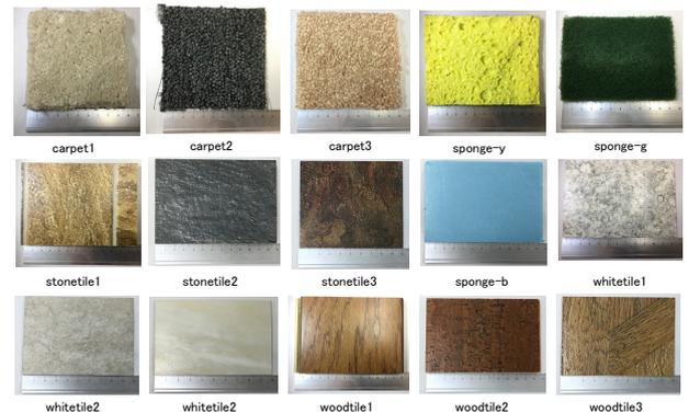
Fig. 5: Textures. These are plate-like object with length 70–100 mm and width 100–130 mm.
