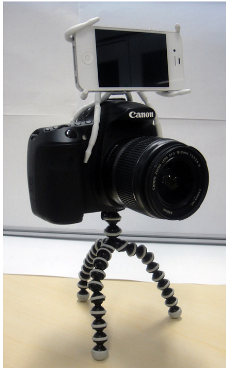
Figure 4.2: Prototype of self-portrait system that use head gestures to make interaction.
