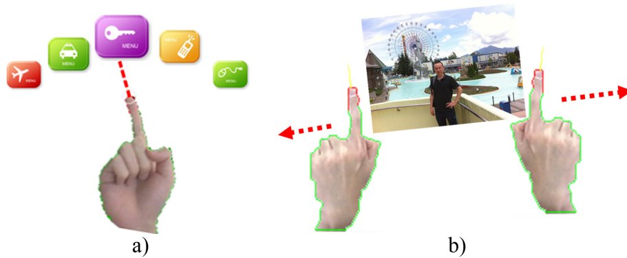
Figure 2.11: The potential user interface design by using hand finger interaction. a) use finger direction as interact approach, b) two hands interface that use to fingers to manipulate of an image.
