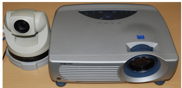
Figure 2 Networked PTZ camera (left) and the beam projector (right)
