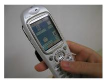
Figure 1. A cellular phone SVNC viewer accessing the desktop of a remote MS Windows system
